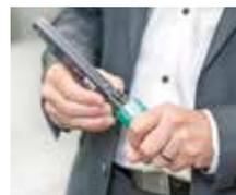
A non-visible taggant is incorporated into the plastic, for example, of a medical device. SICPA's detection pen authenticates original products if the taggant is present. Fakes are identified on the spot with the time and location of the find being relayed online.
